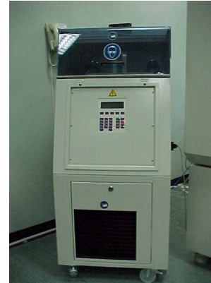
Liquid Thermal Shock Tester Model: Votsch VFS 2/07/15/2
