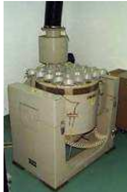
Vibration Test System Model: IMV VS-500-4
