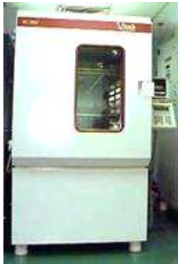
Temperature/Humidity Chamber Model: Heraeus HC7055
