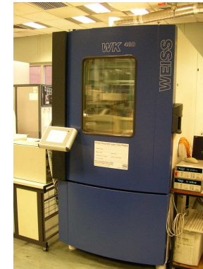
Weiss WK-480/70/15 Climatic Test Chamber Model: Weiss WK-480/70/15
