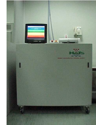
Highly Accelerated Test System (HATS) Model: IRTS
