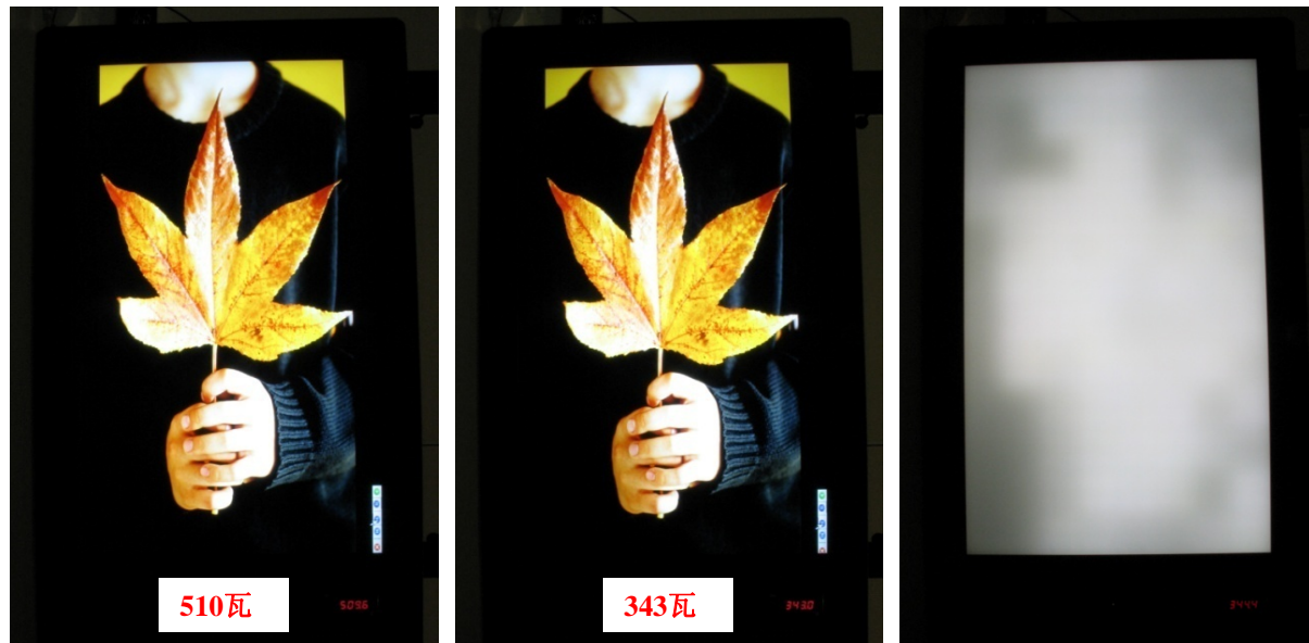
(a) Static LED BLU; (b) dynamic LED BLU, ; (c) Dynamic LED BLU image
